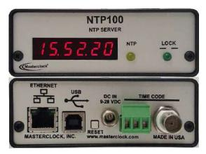
The **NTP100-TC** is an NTP time server that synchronizes to a time code source and converts the signal to Network Time Protocol. It automatically detects the incoming time code source; long-term accuracy is the same as the external source. With loss of time code, the device will revert to an internal oscillator with accuracy of better than 165 msec/day.
